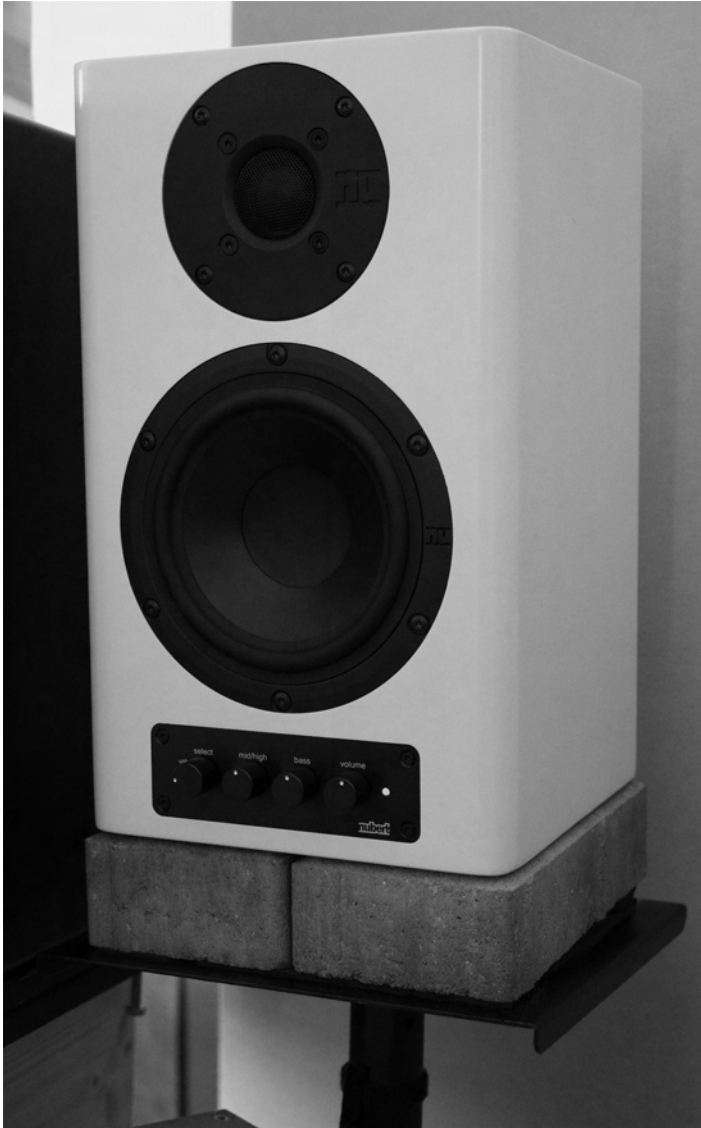
FIGURE 1.6 Resting your nearfield monitors on some heavy bricks or tiles can help increase the speaker cabinet's inertia.
