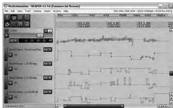
FIGURE 19.9 The vocal level and effect-send automation from a fairly typical Mix Rescue remix. It may look like a lot of data, but that's what it takes to compete in most mainstream musical styles.
